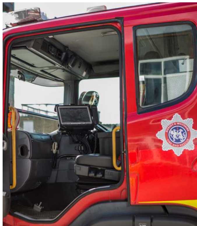
Example installation of the Panasonic CF33 Tablet PC Docking Systems, to a Fire Service Vehicle.
