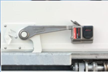
SlamSecure is a heavy duty, mechanical truck and trailer slamlock designed to remove the vulnerabilities and weaknesses associated with conventional commercial vehicle doors.
