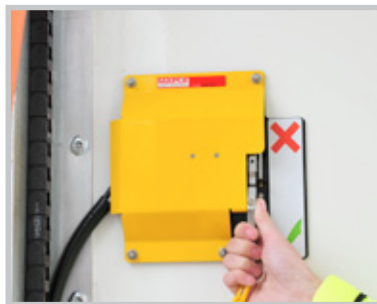
4. With the key in position, air to the brakes is blocked & vented from the brake chambers.
