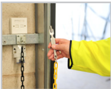
7. With loading complete the key can be removed and returned to the wall mounted bracket.
