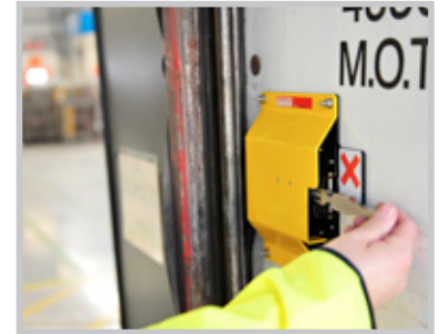
3. Loader inserts the key into the vehicle mounted SafeLoader valve.
