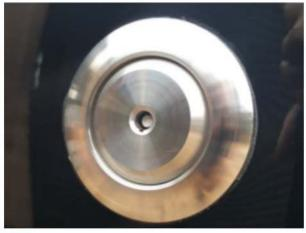
Left: Replock fitted in place of the existing drivers door lock
