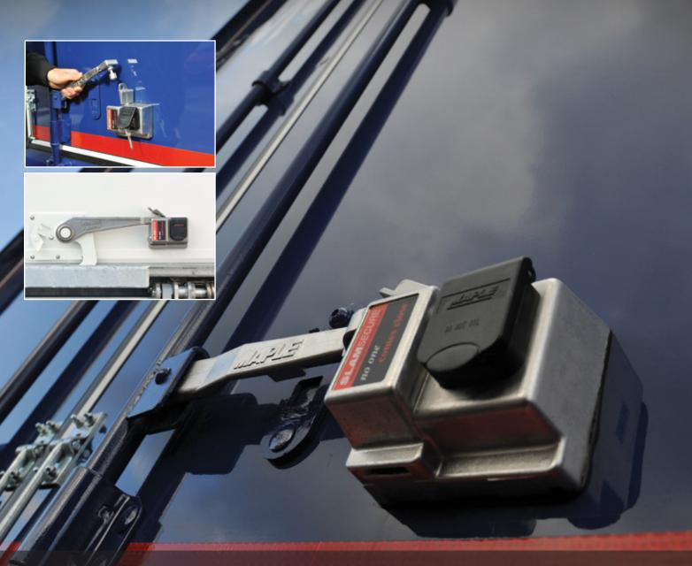
SlamSecure is a heavy duty, mechanical truck and trailer slamlock designed to remove the vulnerabilities and weaknesses associated with conventional commercial vehicle doors.
